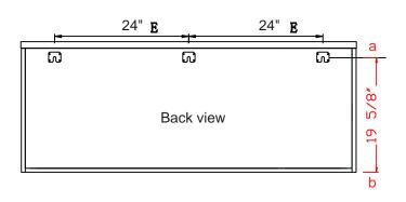
Step 1: Metal plates has been pre-installed to the back of cabinet, Measure the distance between the bottom of the cabinet and point a.
