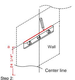
Draw a horizontal line from the point a by using a leveler.
