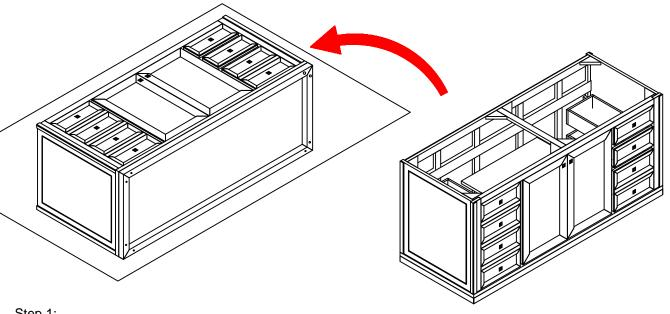
Step 1: To attach the legs, place the cabinet lay down on a blanket or similar soft material.
