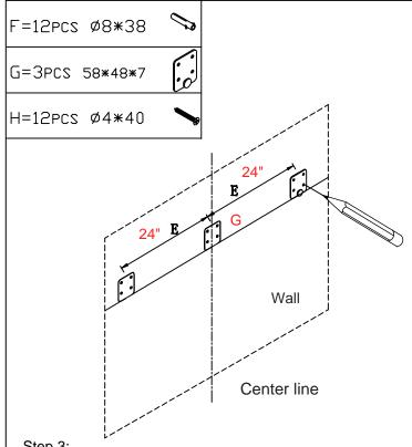
Draw the points according to the hole of the mounting bracket
