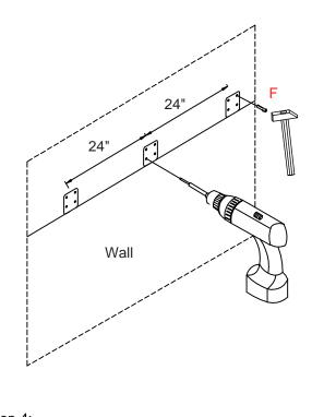
Step 4: Drill the holes' deepth no less than 40mm, and insert "F" to the holes by using hammer.
